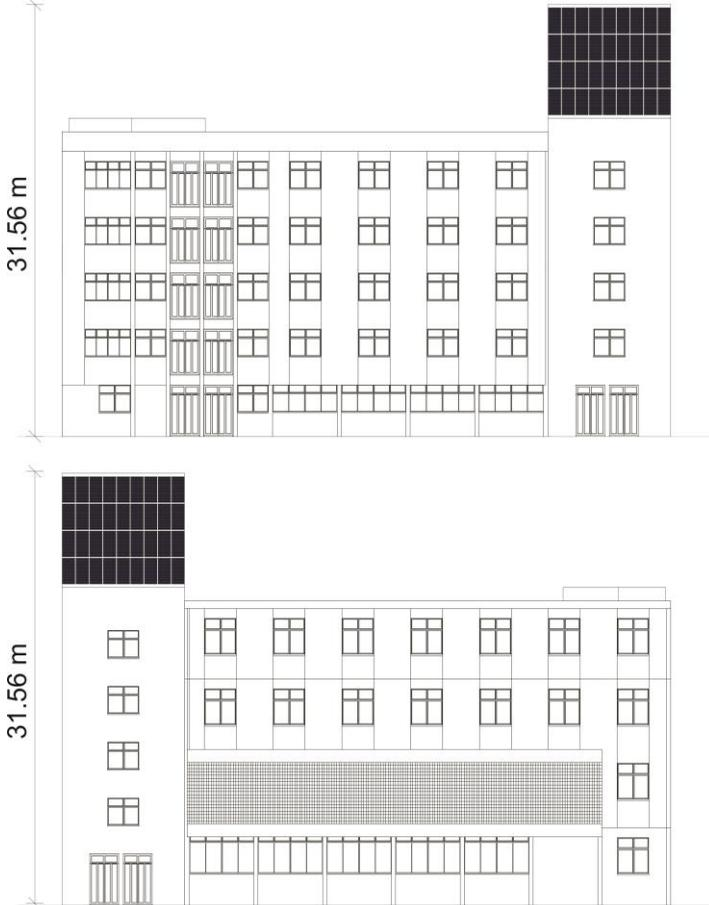
The rooftop integration is composed by 290 PV modules and is shown in Figure 80. The system follows the roof tile’s tilt and orientation.
