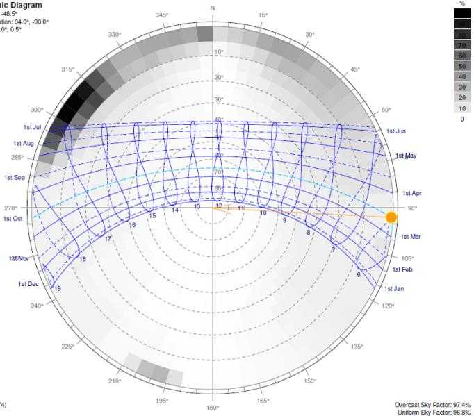
Figure 43 – Building 08’s East surface shading mask.
