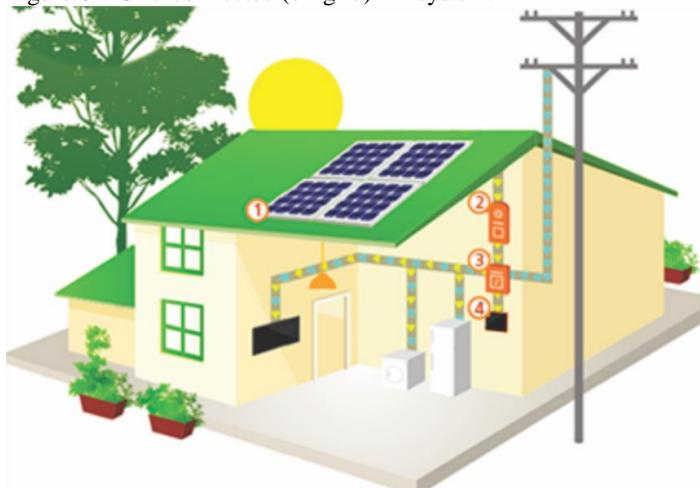
Source: *Tudo Sobre Energia Solar: Tipos de Sistema (On-Grid e Off-Grid)* (ENEL SOLUÇÕES, 2016). Legend: (1) PV modules; (2) inverter; (3) bidirectional counter clock; (4) monitoring.
