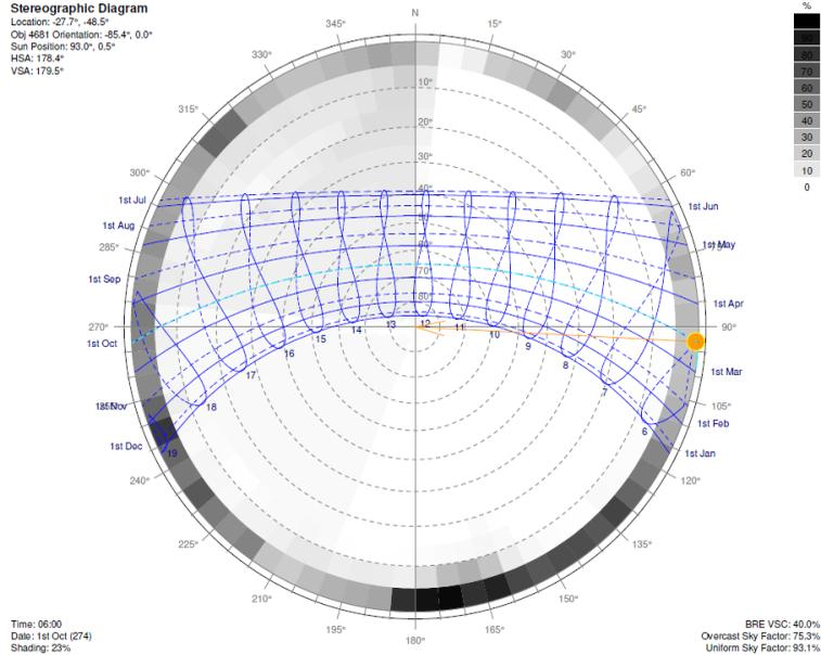
Figure 30 – Building 02’s West surface shading mask.
