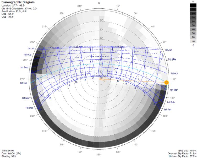
Figure 49 – Building 14’s West surface shading mask.
