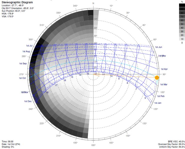
Figure 44 – Building 08’s West surface shading mask.
