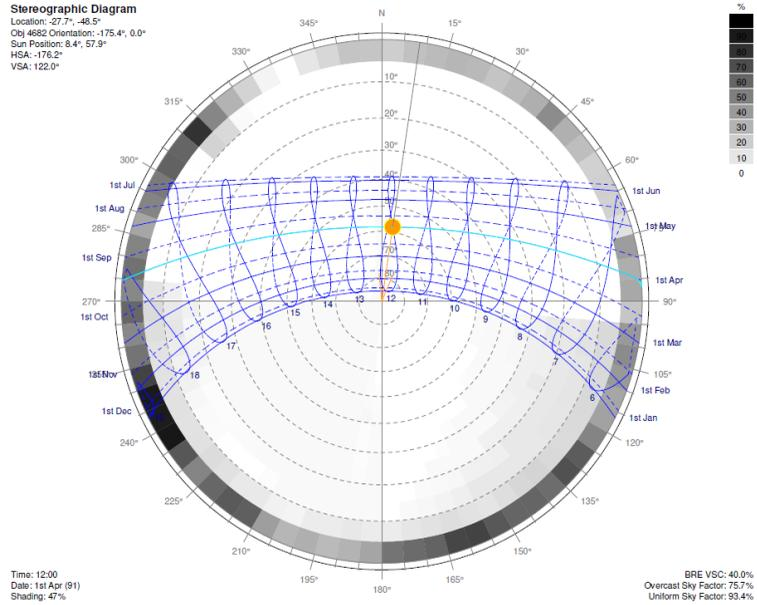
Figure 29 – Building 02’s East surface shading mask.
