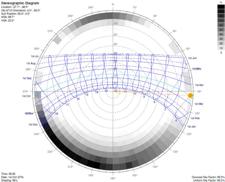
Figure 36 – Building 04’s North surface shading mask.
