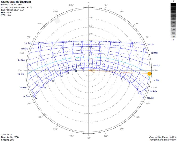
Figure 48 – Building 14’s North surface shading mask.
