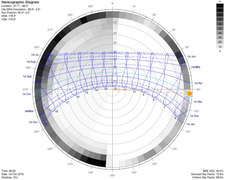
Figure 54 – Building 20’s West surface shading mask.
