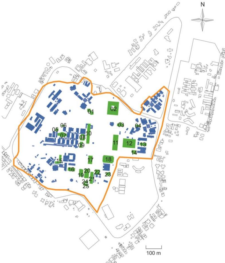
For the Ecotect shading analysis, building 01 was divided in 13 surfaces: 3 rooftops, 3 North surfaces, 3 East surfaces and 4 West surfaces. Only the rooftops (annual shading percentages of 7.7%, 0.1% and 9.2%) and one of the North surfaces (annual shading percentage of 15.6%) were accepted by the shading acceptance criterion.
