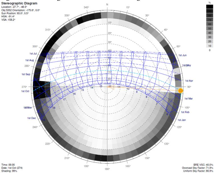
Figure 53 – Building 20’s East surface shading mask.
