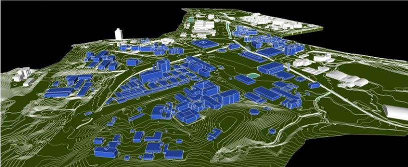
Figure 26 shows the buildings that were considered on the first shading analysis (in green), that is, buildings that have a maximum of  $5^\circ$  azimuthal deviation, and that do not have higher neighboring buildings.
