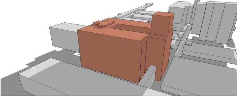
Building 09 was divided in 8 surfaces: 2 rooftops, 2 North surfaces, 2 East surfaces and 2 West surfaces. According to the analysis, one of the rooftops (annual shading percentage of 0.3%) and one of the North surfaces (annual shading percentage of 14.7%) were accepted by the shading acceptance criterion.
