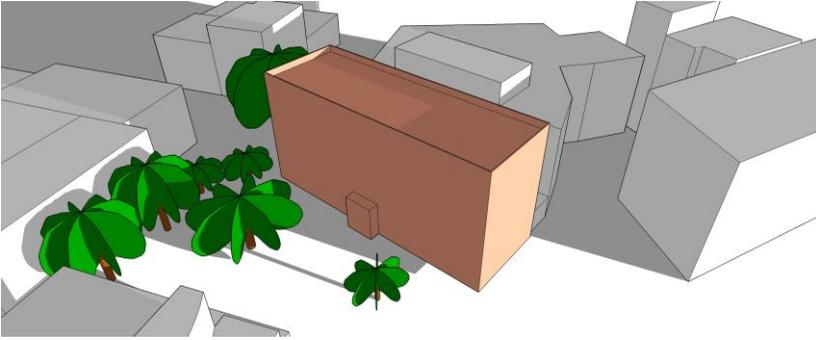
Building 05 was divided in 6 surfaces: 1 rooftop, 2 North surfaces, 1 East surface and 2 West surfaces. According to the analysis, the rooftop (annual shading percentage of 9.5%), one of the North surfaces (annual shading percentage of 10.9%), the East surface (annual shading percentage of 17.3%) and both West surfaces (annual shading percentages of 18.2% and 17.6%) were accepted by the shading acceptance criterion.
