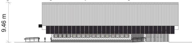
The rooftop integration is composed by 450 PV modules and is shown in Figure 94. The system follows the roof tile’s tilt and orientation.
