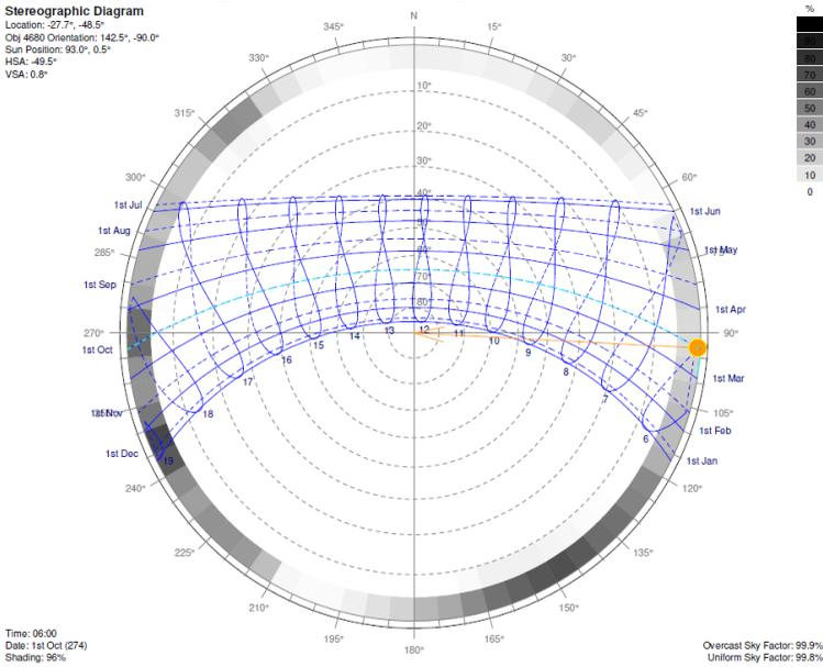
Figure 28 – Building 02’s North surface shading mask.
