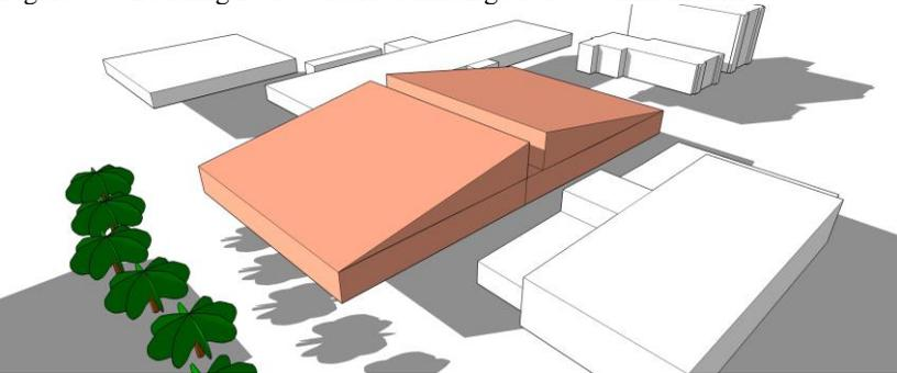
Building 21 was divided in 6 surfaces: 1 rooftop, 1 North surface, 2 East surfaces and 2 West surfaces. According to the analysis, all the surfaces were accepted by the shading acceptance criterion. The rooftop had an annual shading percentage of 6.4%, the North surface of 11.6%,
