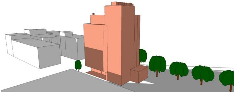
Building 15 was divided in 8 surfaces: 1 rooftop, 2 North surfaces, 2 East surfaces and 3 West surfaces. According to the analysis, the rooftop (annual shading percentage of 2.5%), one of the North surfaces (annual shading percentage of 13.9%) and one of the West surfaces (annual shading percentage of 16.3%) were accepted by the shading acceptance criterion.
