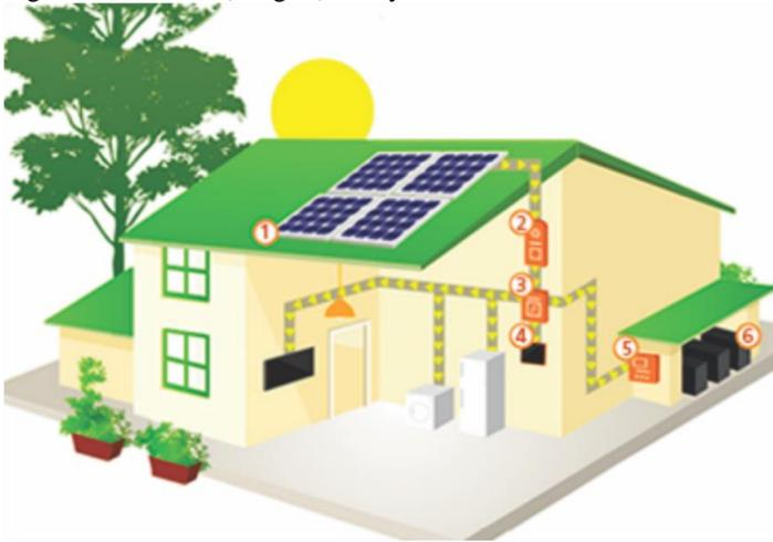
Source: *Tudo Sobre Energia Solar: Tipos de Sistema (On-Grid e Off-Grid)* (ENEL SOLUÇÕES, 2016). Legend: (1) PV modules; (2) inverter; (3) bidirectional counter clock; (4) monitoring; (5) charge controller; (6) battery bank.
