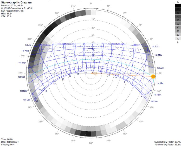
Figure 52 – Building 20’s North surface shading mask.
