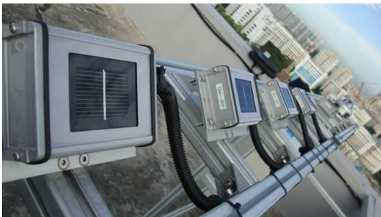
Figure 37: SERIS meteorological station rack, with tilted silicon sensors ranging from 0 to 40 degrees (source: SERIS).
