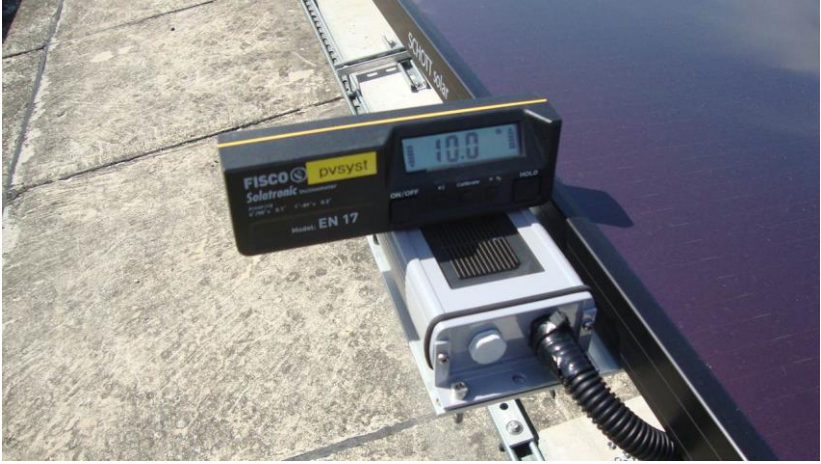
Figure 57: Silicon sensor installed in the plane of the photovoltaic array, here 10 degrees (source: SERIS).
