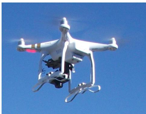
Figure 2 - Aerial IRT-measurement system
