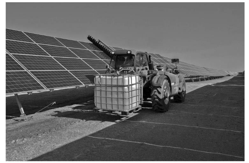
A tractor is used to clean the photovoltaic panels at Finis Terrae solar park near Calama. Strong desert winds stir up dust that coats the panels, reducing their energy output. Tamara Merino/The Washington Post.
